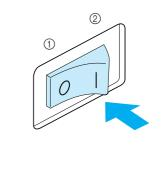
Turn the main power switch to "O" to turn off the machine.
